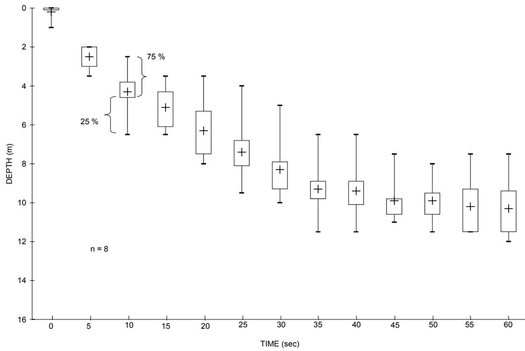
Figure 3. Box plot showing upper and lower quartiles and median (+) hook depth, together with minimum and maximum values (vertical lines) on normal branchlines on the F.V. *Ikatere* (n = 8).
