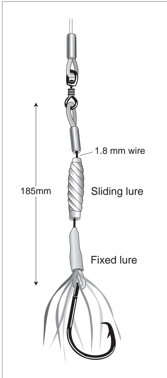
long. The other, experimental branchline was similar but had a fixed and sliding lure on a short, 185-mm wire section on the terminal end of the branchline (Fig. 1). This short wire section increased the overall weight of the branchline by 25 g.
