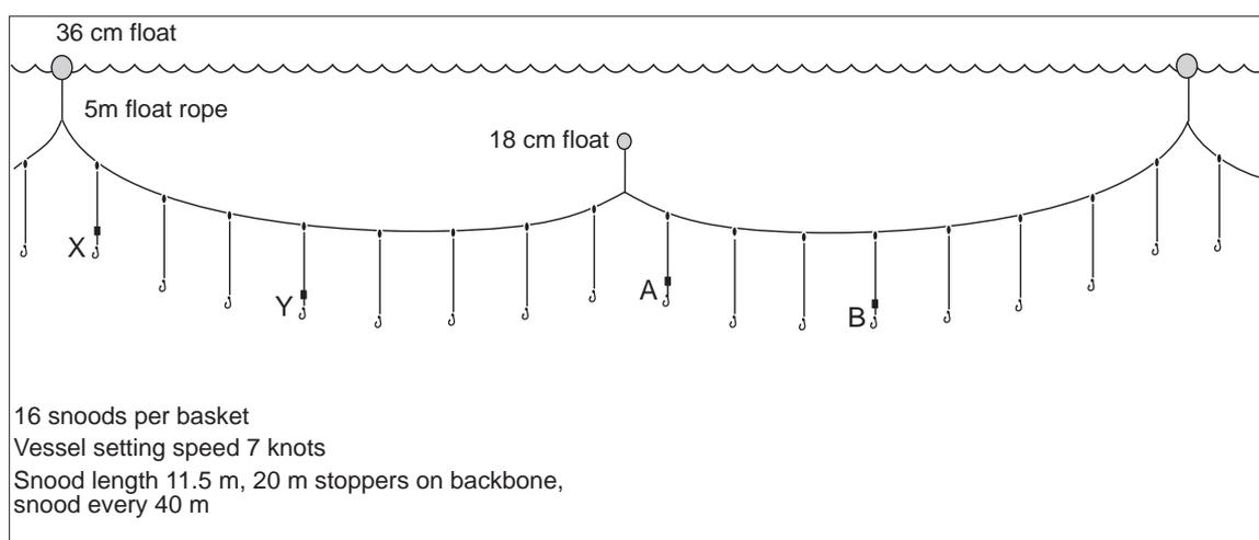
Figure 2. Trial vessel longline configuration (X, Y = TDR positions within one basket; A, B = alternative TDR positions within a subsequent basket).
