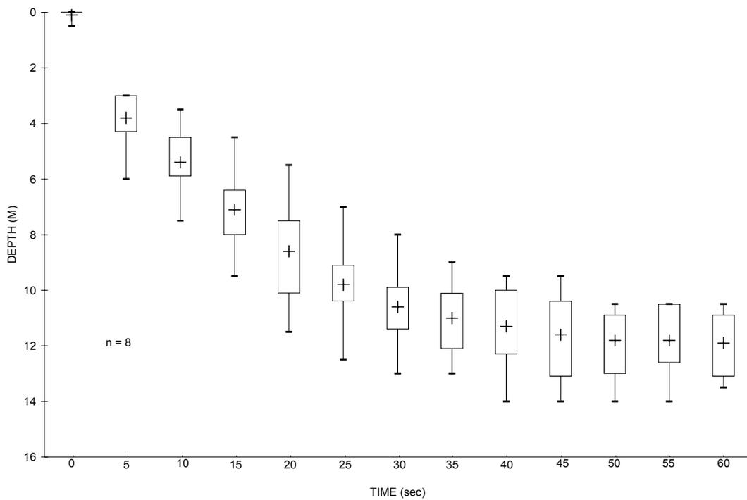
Figure 4. Box plot showing upper and lower quartiles and median (+) hook depth, together with minimum and maximum values (vertical lines) on experimental branchlines on the F.V. *Ikatere*. (n = 8).
